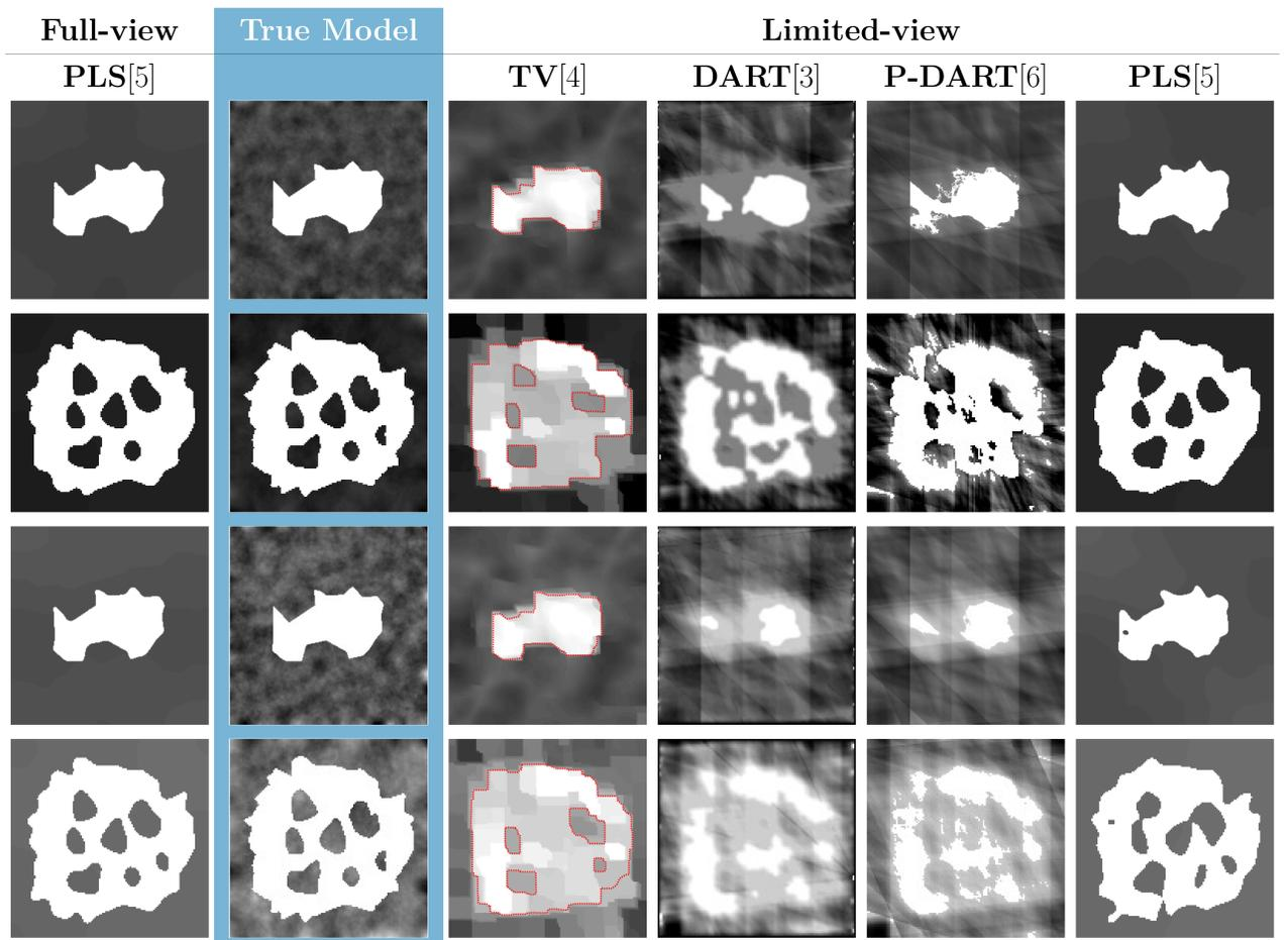
Figure 3: Reconstructions with noisy (SNR=10 dB) full-view ( $\theta \in [0, \pi]$ ) and limited-view ( $\theta \in [0, \frac{2\pi}{3}]$ ) data. All the models have a resolution of  $256 \times 256$  pixels. Full-view: 180 equidistant projections, Limited-view: 5 equidistant projections.
