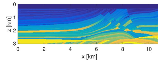
True Marmousi Model discretized on a 20 m x 20 m grid
